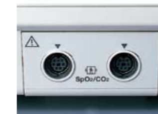
DSI interface unit, QI-552V, for SpO 2 and CO 2 (photo) DSI/AUX out interface unit, QI-553V, for SpO 2 or CO 2 and AUX
